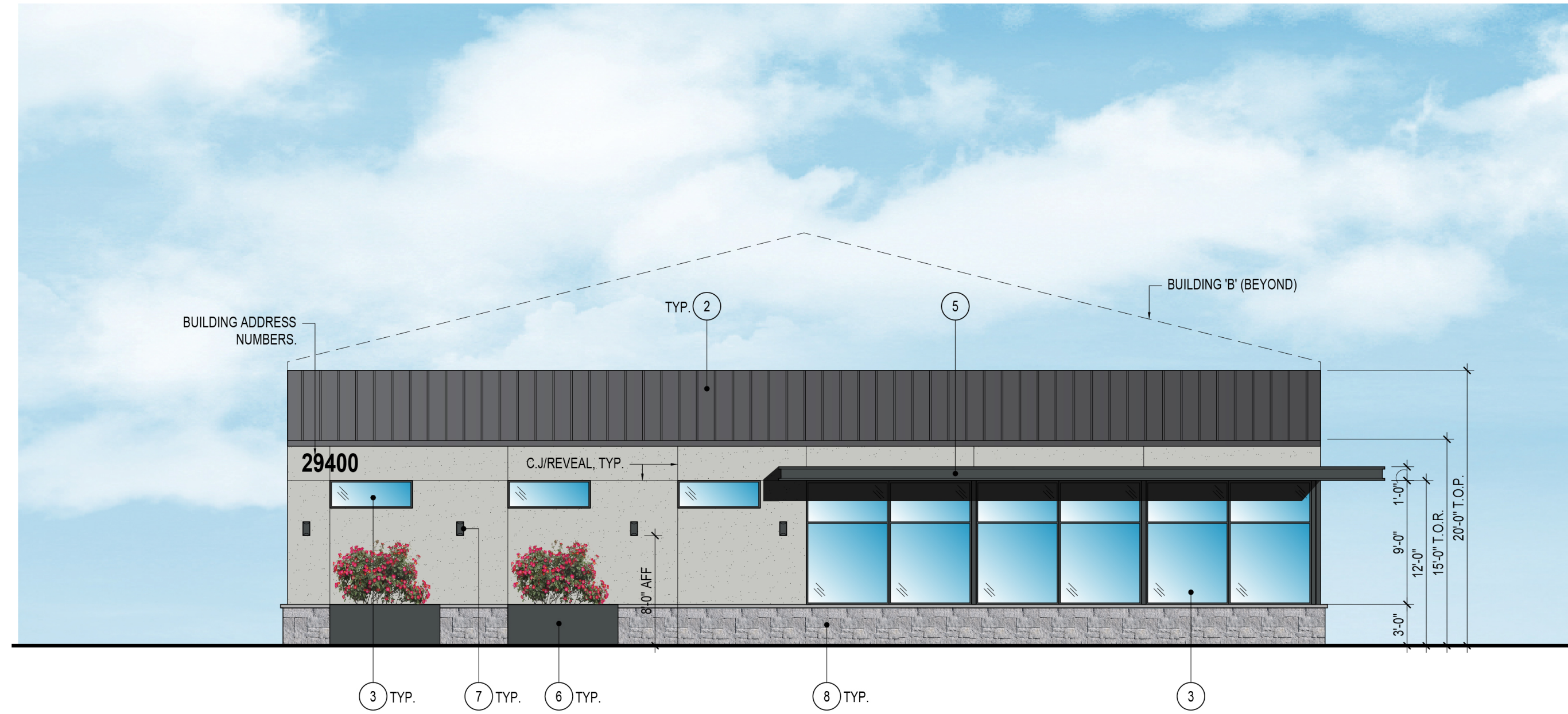
2 FRONT ELEVATION (SOUTH) - BLDG 'A' SCALE: 1/8" = 1'-0"
